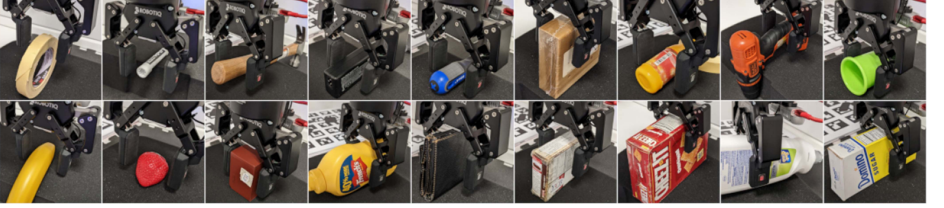
Fig. 1. The objects used for the tactile force tracking and prediction experiments. The relative configuration between the gripper fingers and the object is the one used to perform the experiments before the actual contact takes place.
