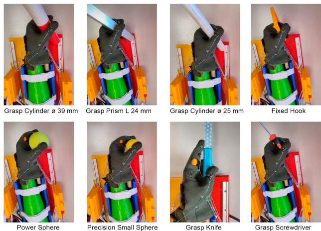
Fig. 8. Exoskeleton tasks during tests.
