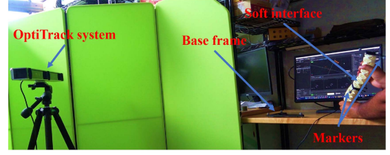
Fig. 4. Capturing human demonstrations while moving the flexible interface with Motion Capture System.
