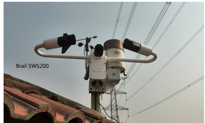
Fig. 4. Brail SWS200 placed 3 m above ground.
