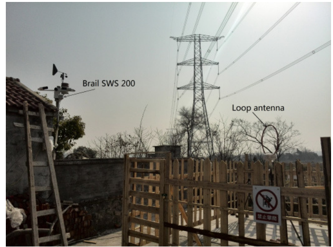
Fig. 3. Loop antenna placed below midspan, 20 m lateral.
