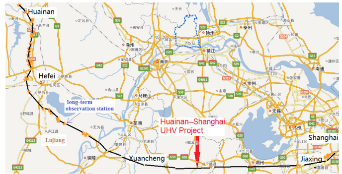
Fig. 1. Chinese Huainan–Shanghai 1000 kV UHV AC double-circuit transmission line.
