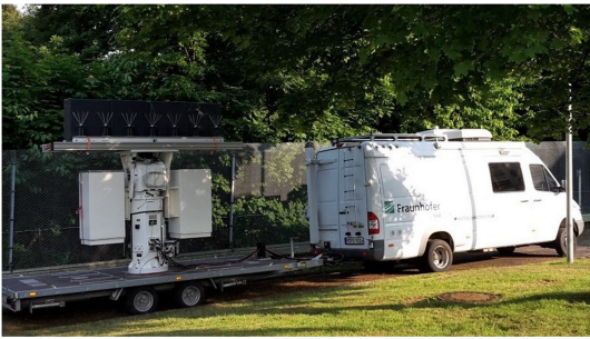
Fig. 13. Experimental multichannel receiver mounted on the back of a van in a side-looking configuration.
