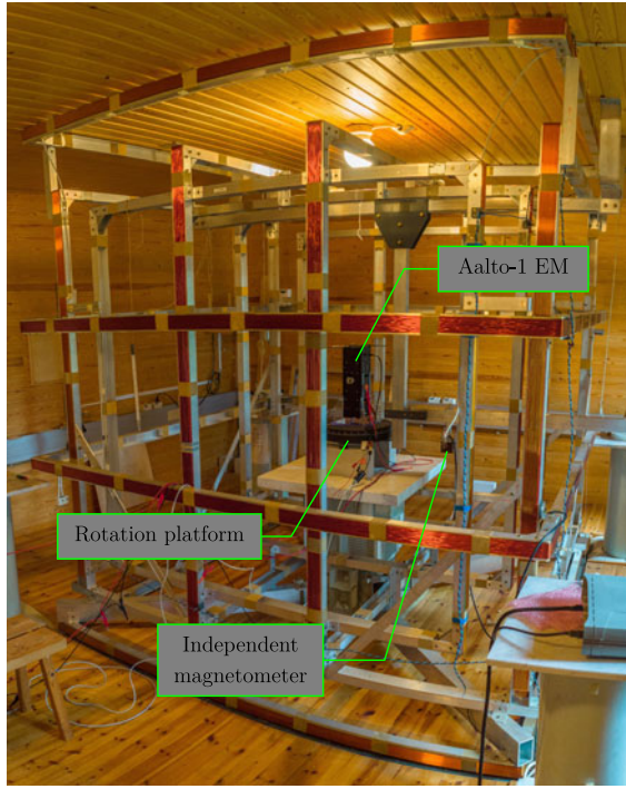
Fig. 6. Magnetic test facilities with Helmholtz cage setup in Nurmijärvi Geophysical Observatory, operated by Finnish Meteorological Institute. The specifications of the test setup are available in [34].
