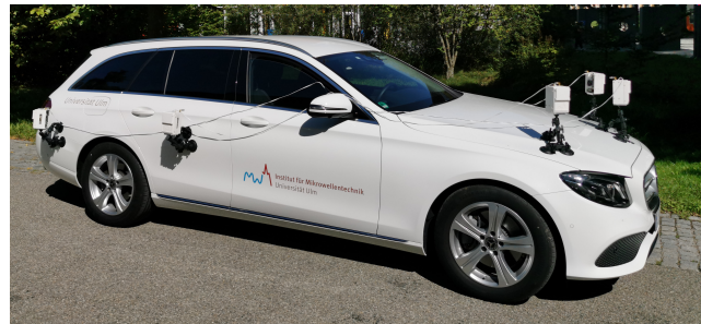
Fig. 4: Experimental system setup with seven chirp-sequence radar sensors mounted on a car.
