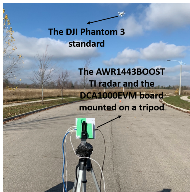
Fig. 19: Measurements setup of the DJI Phantom 3 standard quadcopter.
