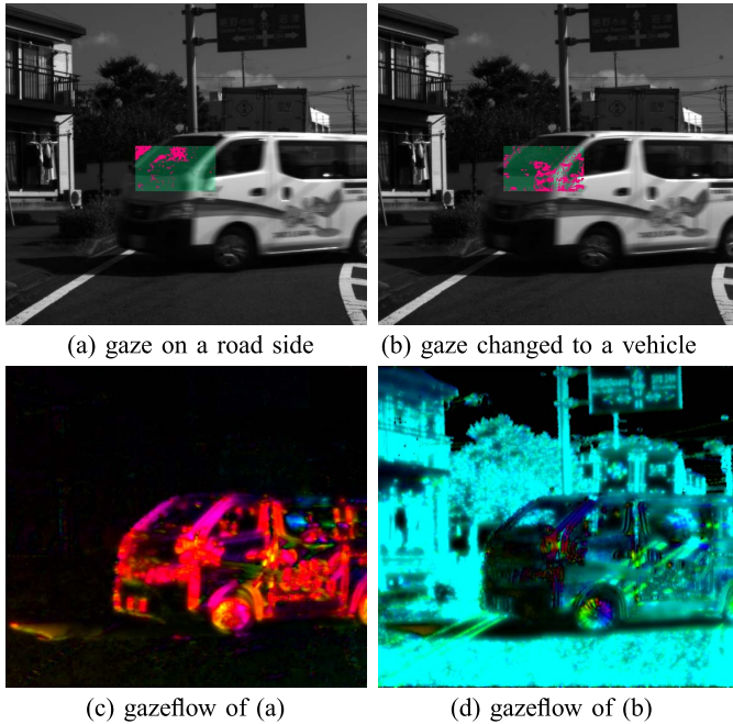
Fig. 14. Induced transition of the gaze target to a vehicle crossing in front. (a) and (b) gaze areas (red) in gaze rectangles (cyan) before and after the transition, (c) and (d) gaze-flows for (a) and (b). In (a), the gaze target was on the left and through the window of the vehicle, and the gaze-flow (c) captures the leftward motion of the crossing vehicle. In (d), relative motions in the vehicle (wheel rotation and surrounding reflection) become more evident.
