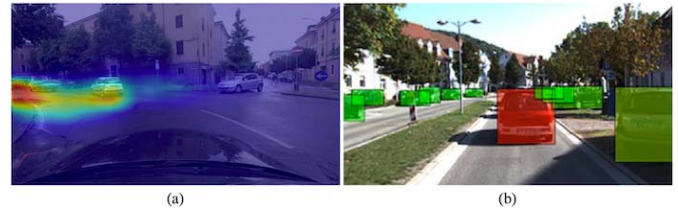
Fig. 6. Sample outputs of driver gaze estimation algorithms. a) Pixel-level saliency map for vehicle performing a left turn. b) Visualization of object-level importance scores for vehicle following. Red color indicates higher relevance/importance in both images. Sources: a) [198], b) [201].
