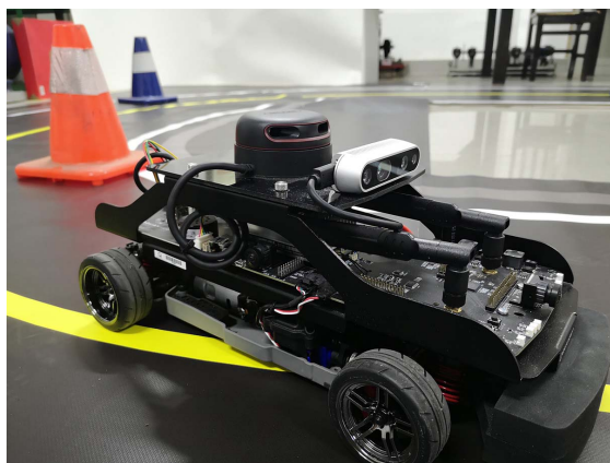
Fig. 11. QCar: a small-size autonomous vehicle platform.
