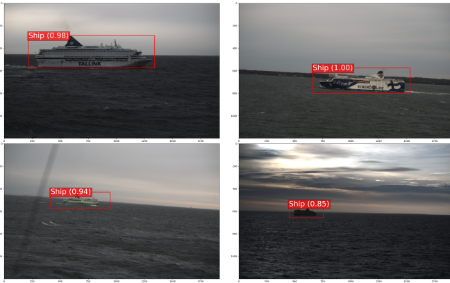
Fig. 8. Experiments of vision-based ship recognition conducted on board MS Megastar . The rectangle box gives the location and label of detection. The number in parenthesis is the confidence of detection. The images are challenging to detect, as they have low brightness and ill exposure problems.
