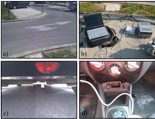
Fig. 18. (a) Magnetic loops. (b) Test material. (c) RFID card in the rear part of the vehicle. (d) Mains socket.
