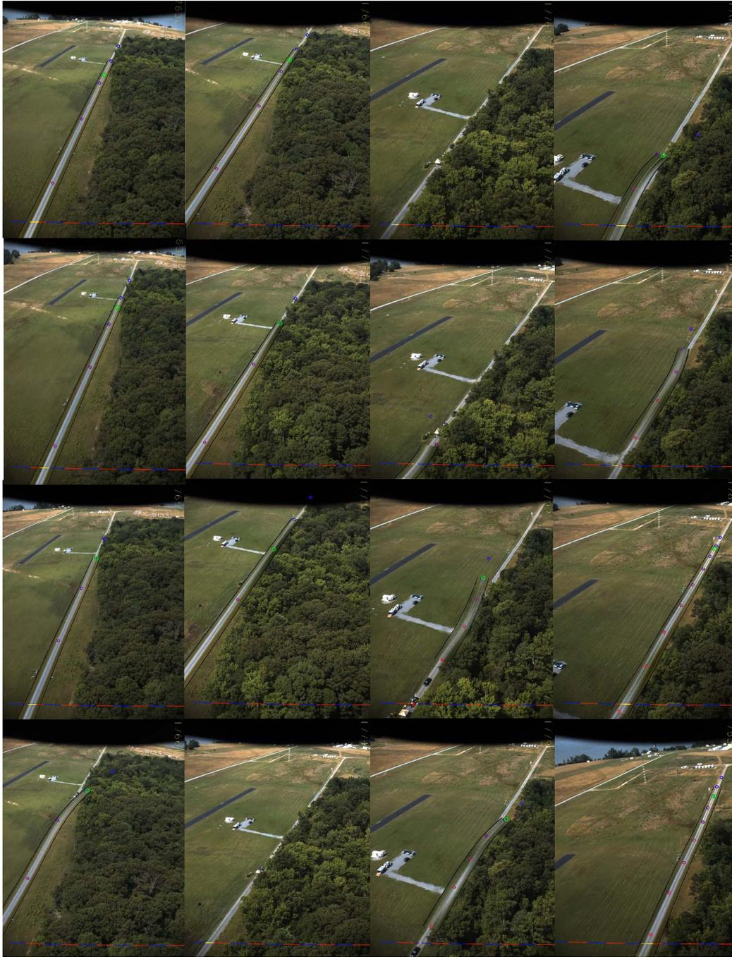
Fig. 8. This a sequence of images showing the view seen by the aircraft during a short period of an actual test flight. The road model generated by the aircraft, which is the detected road, is overlaid on the images. The images show the impact of a tree canopy occluding the road at various degrees. The flight is not impacted significantly as the aircraft rediscovers the road.
