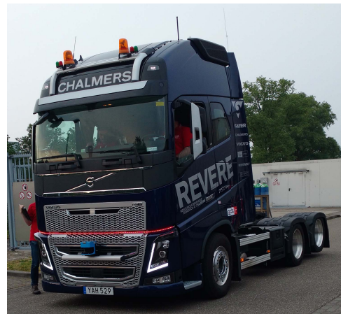
Fig. 2. The external HMI is exemplified on a truck. The light bar is showing red light for evaluation purposes; see the text for a description of the behavior.
