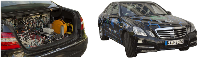
Fig. 2. Bertha , the flagship automated vehicle of Team AnnieWAY.
