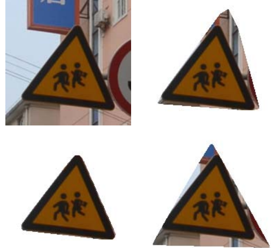
Fig. 3. Segmentation results with varying parameter r . Top left: source region of interest containing a triangle sign. Top right: r = 2 . With this setting, the shape term is always weaker than the smoothness term, so segmentation is dominated by contrast. Bottom left: r = 4 . The color term now plays a more important role in earlier iterations while the shape term dominates the energy in later iterations. Segmentation converges to the desired result. Bottom right: r = 8 . The shape term dominates the energy too soon and iteration fails to converge to the correct segmentation.
