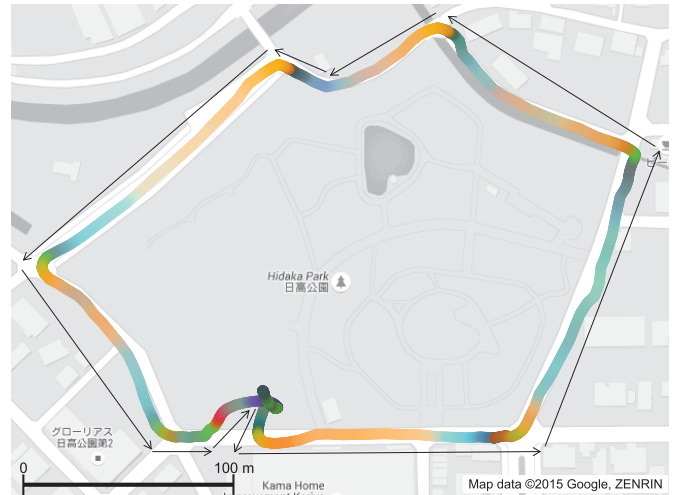
Fig. 9. Visualization result of the driving behavior on the public road around Hidaka Park by using the trained DSAE.
