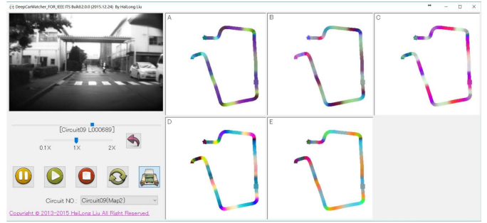
Fig. 4. The modified version of Deep Car Watcher for subjective evaluation, which shows driving videos and the driving color maps obtained using PCA (A), FastICA (B), KPCA (C), SAE (D), and DSAE (E). This software does not show the name of the methods, but instead it indicates them as A~E to label the driving color maps.
