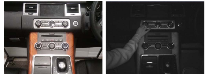
Fig. 1. Control panel. (Left) Under normal lighting conditions with an RGB camera. (Right) With a near-infrared camera with near-infrared illumination.
