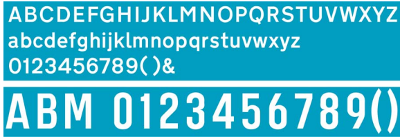
Fig. 17. U.K. traffic sign typefaces, showing (top) transport typeface and (bottom) motorway typeface.
