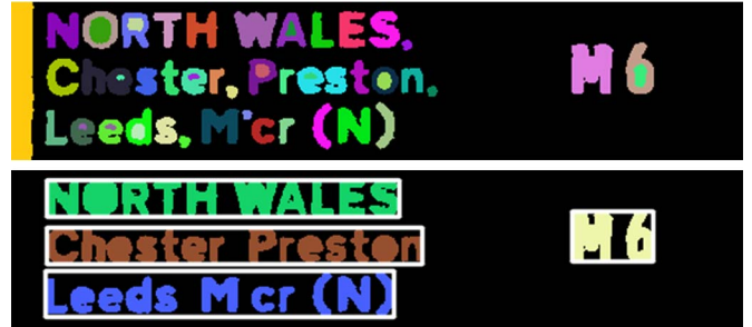
Fig. 15. Stages of line detection, showing (top) detected MSERs and (bottom) detected text lines.
