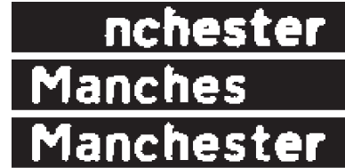
Fig. 19. Combination of word fragments, showing (top and middle) two word fragments and (bottom) the resulting combination of those word fragments.
