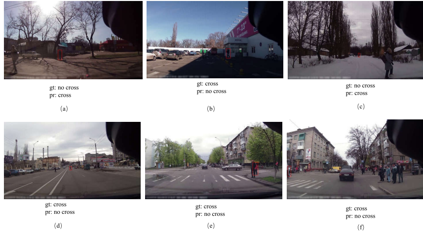
Fig. 6. Typical examples of detection failures. 'gt' is the ground truth classification value, and 'pr' is the predicted value. The illumination, remote distance, and occlusion of obstacles are the main reasons for failure detections.
