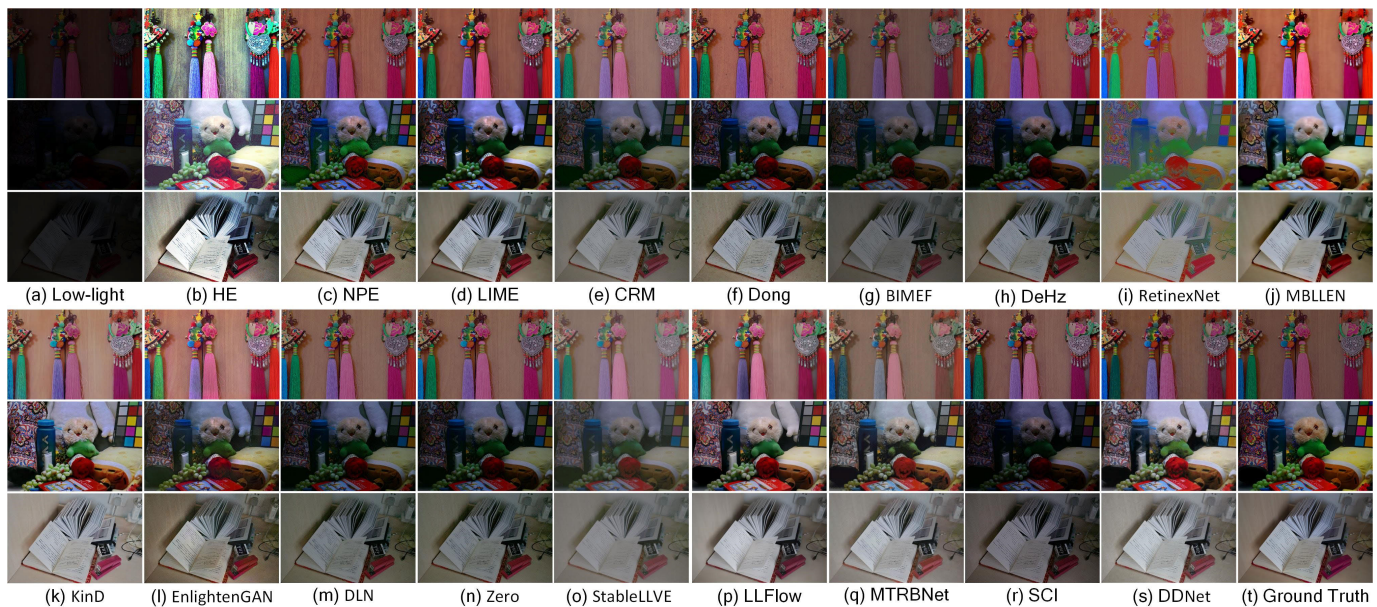
Fig. 7. The visual comparisons of different enhancement methods for three typical images from the LOL dataset [36]. From left to right: (a) Low-light images, restored images, generated by (b) HE [16], (c) NPE [26], (d) LIME [27], (e) CRM [29], (f) Dong [31], (g) BIMEF [30], (h) DeHz [32], (i) RetinexNet [36], (j) MBLLEN [40], (k) KinD [35], (l) EnlightenGAN [46], (m) DLN [41], (n) Zero [22], (o) StableLLVE [42], (p) LLFlow [43], (q) MTRBNet [44], (r) SCI [23], (s) the proposed DDNet, and (t) Ground Truth, respectively.
