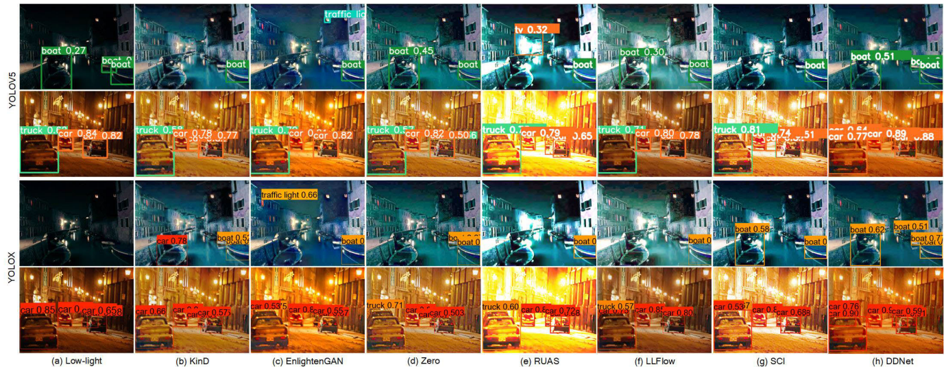
Fig. 9. The qualitative results of object detection experiments on low-light transportation surveillance data, which select YOLOv5 and YOLOX [3] as the basic detection methods. From left to right: (a) Low-light images, the enhanced images of (b) KinD [35], (c) EnlightenGAN [46], (d) Zero [22], (e) RUAS [37], (f) LLLFlow [43], (g) SCI [23], and (h) the proposed DDNet, respectively. It can be seen that DDNet is more beneficial for detection accuracy improvement due to the enhancement of edge features on the gradient domain.
