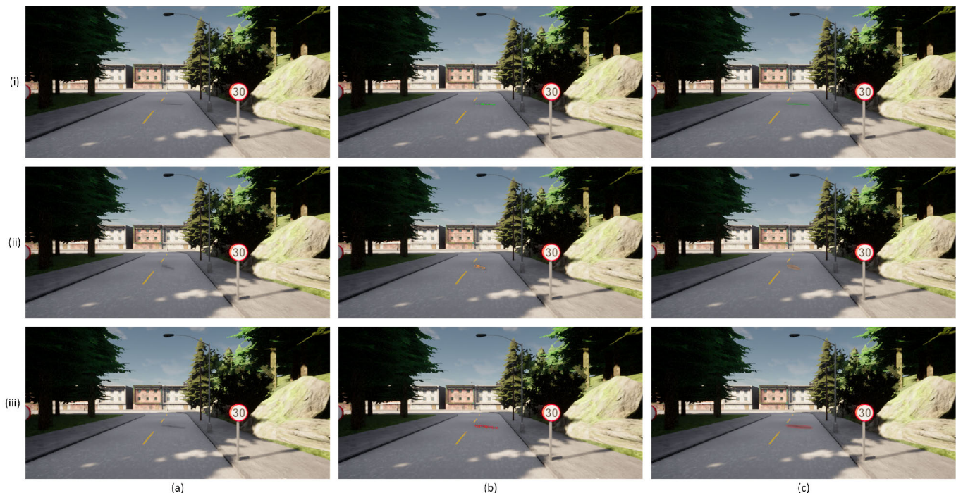
Fig. 9. (i-iii) Different severity prioritization of potholes based on their size and volume, (a) image of the camera without any visual cue, (b) projected point cloud representing the identified pothole, (c) overlay visualization of the pothole.
