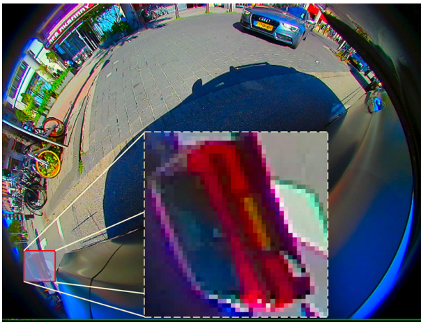
Fig. 6. Zoomed-in segment of a Woodscape dataset image showing evidence of lateral chromatic aberration. Note the slight red/purple and green tint in the pixels along the outline of the car and the road marking.
