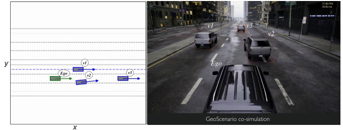
Fig. 1. A challenging interaction between ego and human-operated vehicles based on a pre-crash scenario from NHTSA [2] and using our SDV model in simulation: (left) in the map frame, the SDV Model as v_2 performs the cut-in maneuver targeting ego, and (right) a high-fidelity co-simulator renders the scene.
