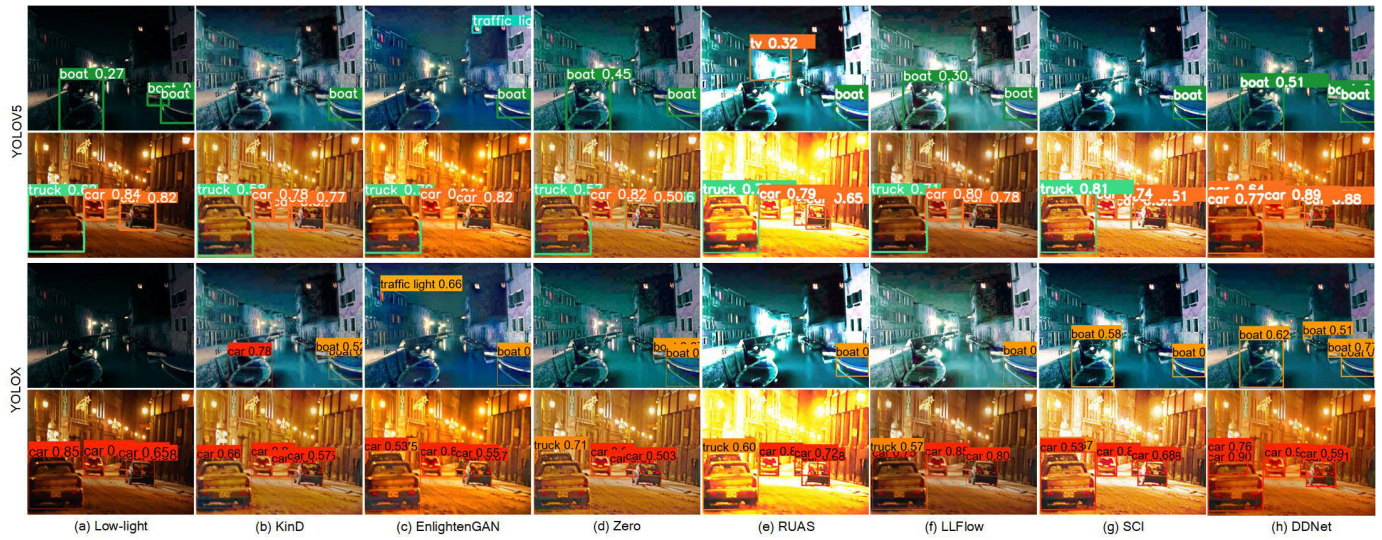
Fig. 9. The qualitative results of object detection experiments on low-light transportation surveillance data, which select YOLOv5 and YOLOX [3] as the basic detection methods. From left to right: (a) Low-light images, the enhanced images of (b) KinD [35], (c) EnlightenGAN [46], (d) Zero [22], (e) RUAS [37], (f) LLFlow [43], (g) SCI [23], and (h) the proposed DDNet, respectively. It can be seen that DDNet is more beneficial for detection accuracy improvement due to the enhancement of edge features on the gradient domain.
