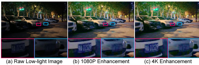
Fig. 2. The comparison between the low-light enhancement results on UHD images in transportation surveillance. From left to right: (a) raw 4K low-light image, (b) enhanced result after resizing the image to 1080P, and (c) 4K image enhancement. It is obvious that the resizing operation causes significant detail loss on UHD images.
