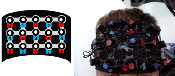
Fig. 2. Channels montage and representation of the whole setup device –in our case, the hardware was placed behind the passenger seat.
