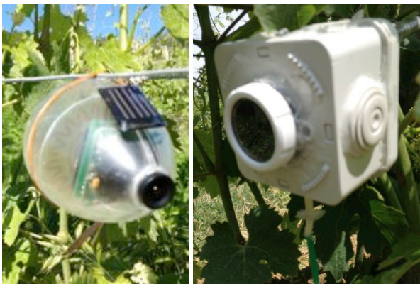
Fig. 9. Two SNs installed in a vineyard. Left: with internal harvester, right, with external harvester
