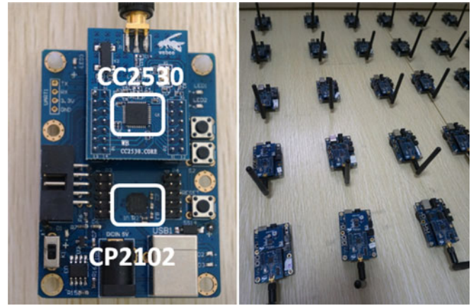
Fig. 6. Node devices of the experimental IoT network.
