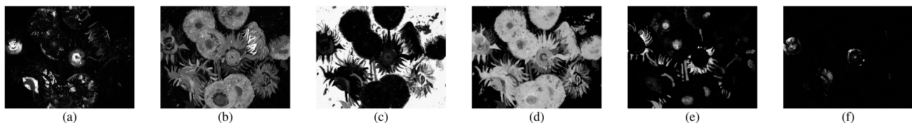
Fig. 10. Quantity maps of the major emission line groups of example chemical element produced using Bruker M6 software (after deconvolution) for the scanned region of Sunflowers . (a) Iron (Fe) K_{\alpha} , (b) Chromium (Cr) K_{\alpha} , (c) Zinc (Zn) K_{\alpha} , (d) Lead (Pb) L_{\beta} , (e) Copper (Cu) K_{\alpha} , and (f) Bromine (Br) K_{\alpha} .
