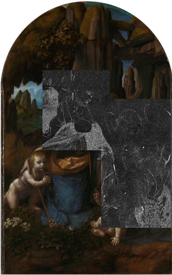
Fig. 18. Combined Zn K_{\alpha} quantity map produced by our algorithm for the three scanned regions of ‘ The Virgin of the Rocks ’, revealing underdrawing related to an abandoned earlier composition.
