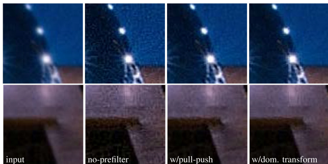
Fig. 9. Pre-filtering. When the input image presents noise and other artifacts, Polyblur can amplify artifacts. As a pre-step, we may apply any filter that separates high-frequency texture and other details [56], [57], apply Polyblur ( \alpha = 6 , b = 1 ), and finally add back the residual.
