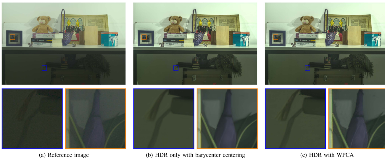
Fig. 6. Use of the weighted principal components permits to increase detail and texture preservation.
