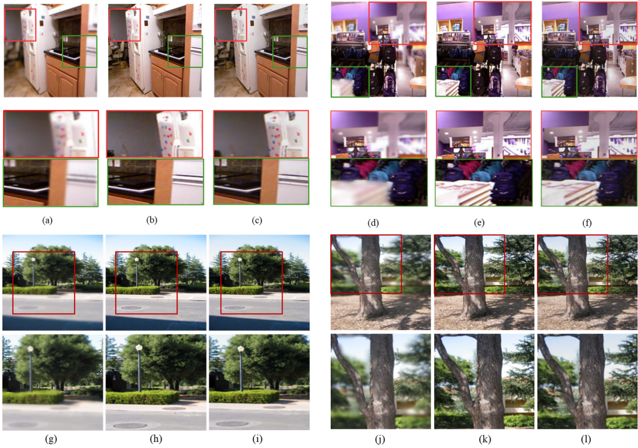
Fig. 8. 2HDED:NET results for deblurring on NYU-v2 and Make3D dataset. From left to right: (a) defocused image, (b) ground truth AiF image, and (c) deblurred image. Similarly, (d), (e), and (f) for a different scene. Zoomed-in patches are shown below each scene.
