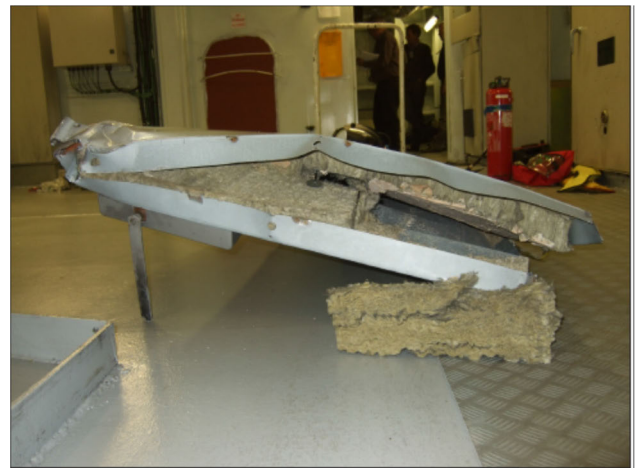
FIGURE 18. Steel door from harmonic filter capacitor bank on Queen Mary II REF SB4-10.
