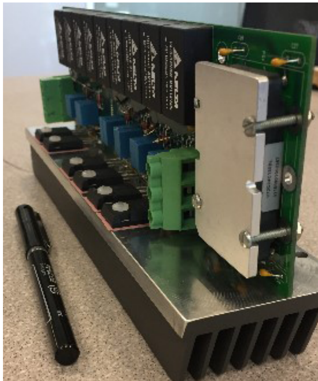
FIGURE 1. Picture of the prototype 2kW 208V (240V) three-phase single-stage boost CSI.
