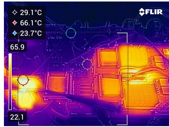
Fig. 10. Thermal test results at 2200 W under natural convection cooling.
