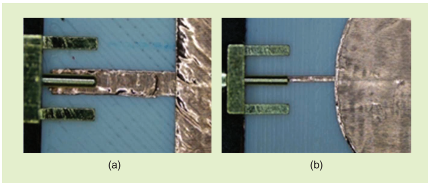
Figure 3. Digital microscope photos of the connector connection (no solder). (a) Rectangular patch. (b) Circular patch.
