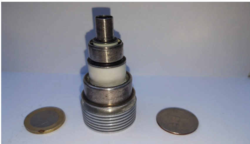
Figure 1. The 2C39 (3CX100A5) UHF triode (U.S. quarter and Euro for scale).
