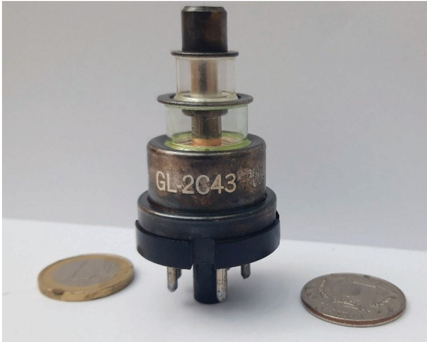
Figure 4. A 2C43 triode capable of generating 3 kW of pulsed power at 3 GHz.
