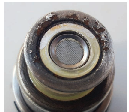
Figure 3. An internal view of a 2C43 triode at the grid ring level.
