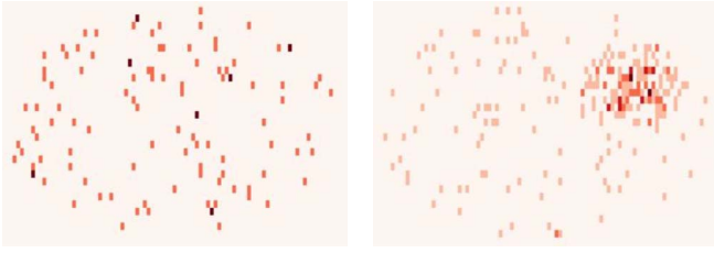
Fig. 1. Defect density wafer map with the random defects (left) and with the random and the non-random defects (right).
