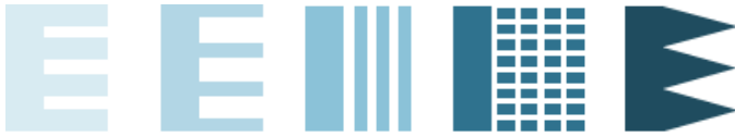
Fig. 3: Examples of the geometrical shapes used in the PSR mark designs. The large process insensitive zone is on the left of each design, and the process-sensitive finely patterned zone is shown on the right.
