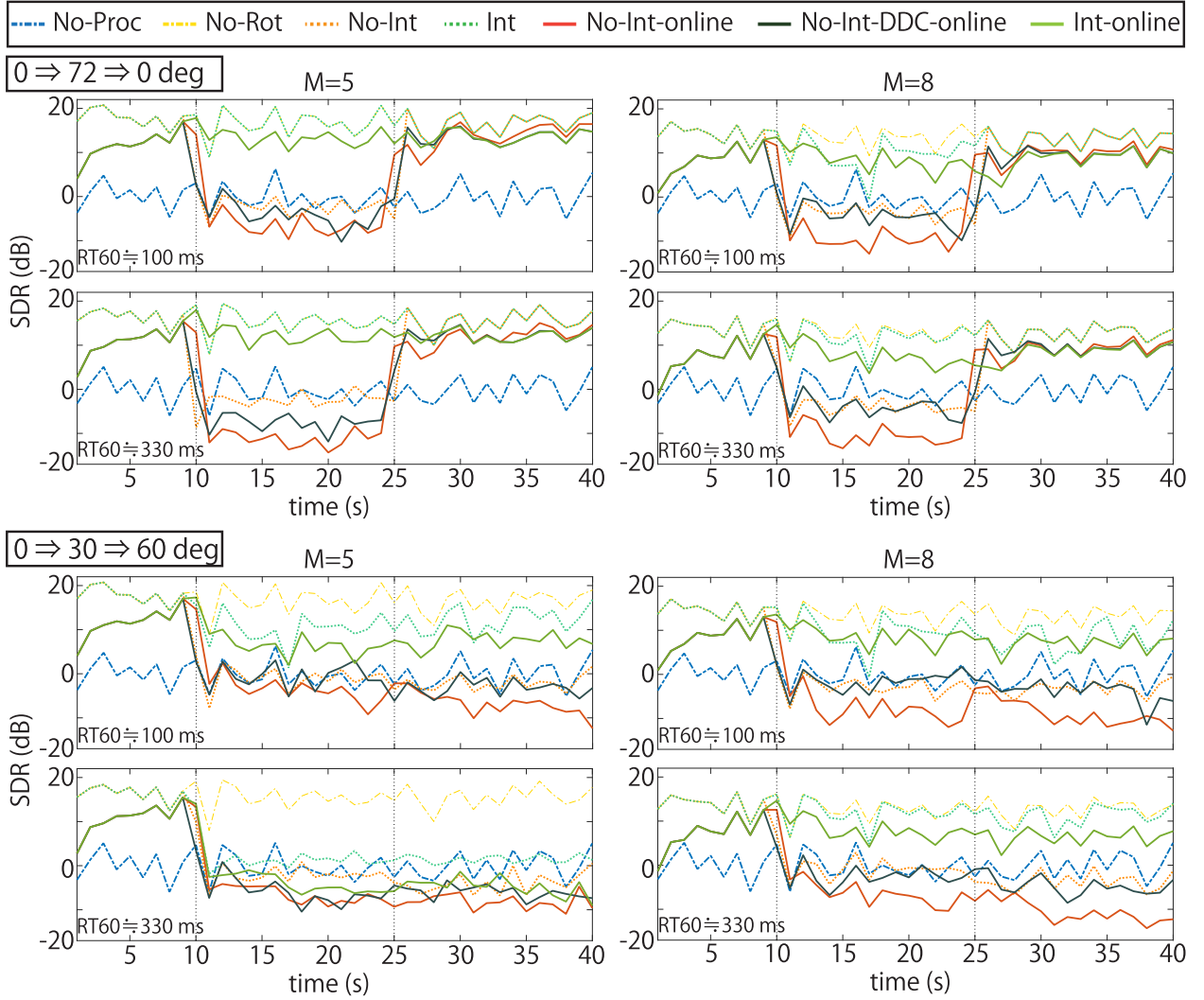
Fig. 11. Segmental SDR every 1 s with M = 5 and 8 and RT60 = 100 and 330 ms, where the two vertical dashed lines indicate the time points when the rotation occurred with the two patterns: 0 \Rightarrow 72 \Rightarrow 0 deg and 0 \Rightarrow 30 \Rightarrow 60 deg. No-Proc shows the mixture itself, No-Rot shows the case where rotation does not occur, No-Int and Int respectively show batch processing without/with interpolation, DDC indicates that the SCM is updated in direction-dependent manner, and -online shows online processing with the smoothing factor \alpha of 0.99 .
