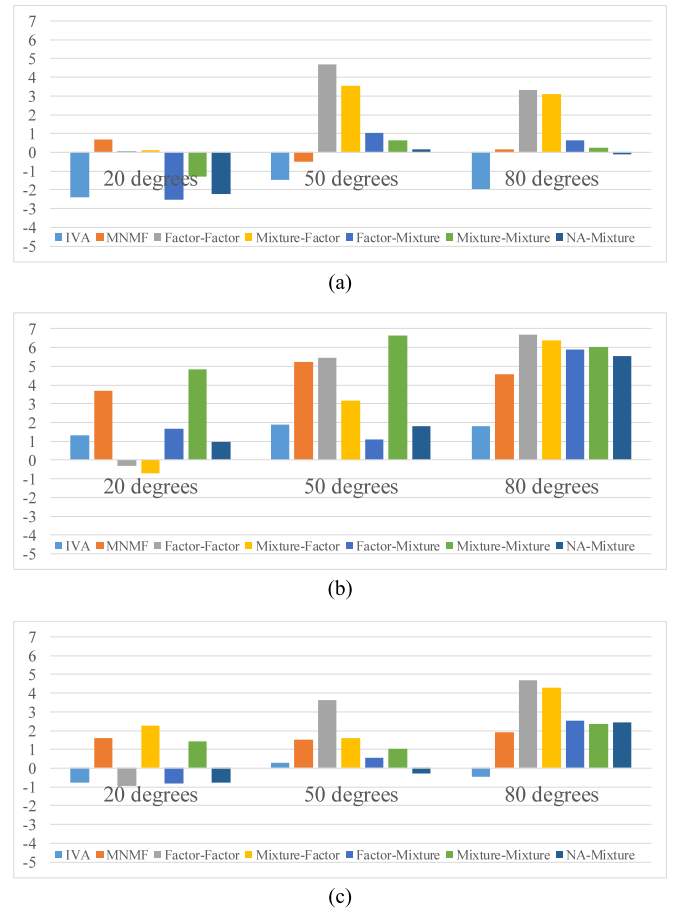
Fig. 16. The SDRs obtained by IVA, MNMF, and the factor-factor, mixture-factor, factor-mixture, mixture-mixture, and spatial-mixture models for the inter-source interval of 20°, 50°, and 80°. (a) Music mixtures. (b) Speech mixtures. (c) Music and speech mixtures.
