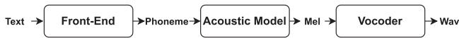
Fig. 1. System diagram of a typical TTS synthesis pipeline. Mel refers to the acoustic feature Mel-spectrogram, while Wav is the speech waveform.
