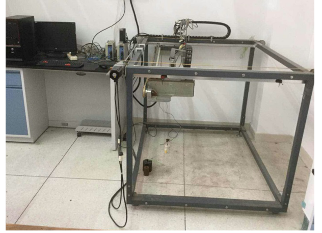
Fig. 2. Self-built scaled crane testbed.
