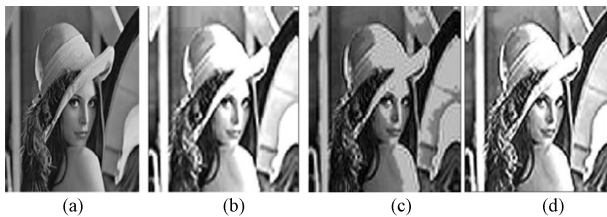
Fig. 8. (a) Original low-contrast image. (b) Enhanced image with \alpha = 0.29 . (c) Enhanced image with \alpha = 0.4 . (d) Enhanced image with \alpha = 0.53 .
