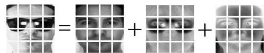
Fig. 2. Local sparse representation. The query image is divided into several blocks. The first image is the query image; the second image is recovered by the gallery set; the third is represented by the external data; the last is the representation residual.
