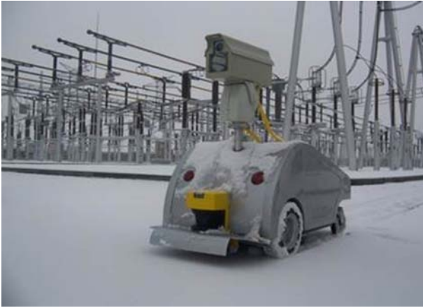
Fig. 1. Power substation inspection robot developed by Electric Power Robotics Laboratory.
