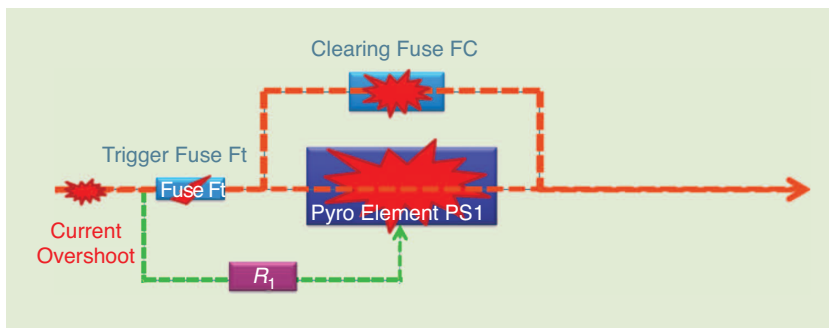
FIG 2 The fuse in series is underrated versus the voltage of the application. It is designed to act at an overcurrent high enough to prevent spurious tripping. (Figure courtesy of Mersen.)
