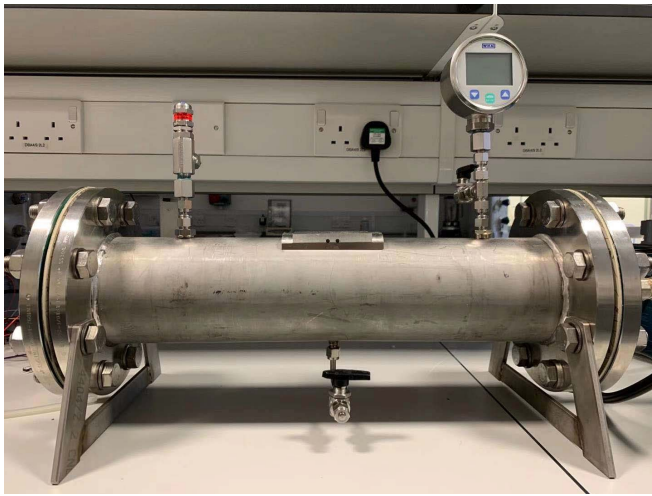
Fig. 11. Static pressure test rig.
