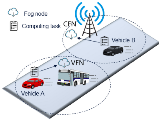
Fig. 1. Application scenario of VFC, where Vehicle A offloads its task to a VFN carried by a bus and Vehicle B offloads its task to a CFN co-located with a cellular BS.
